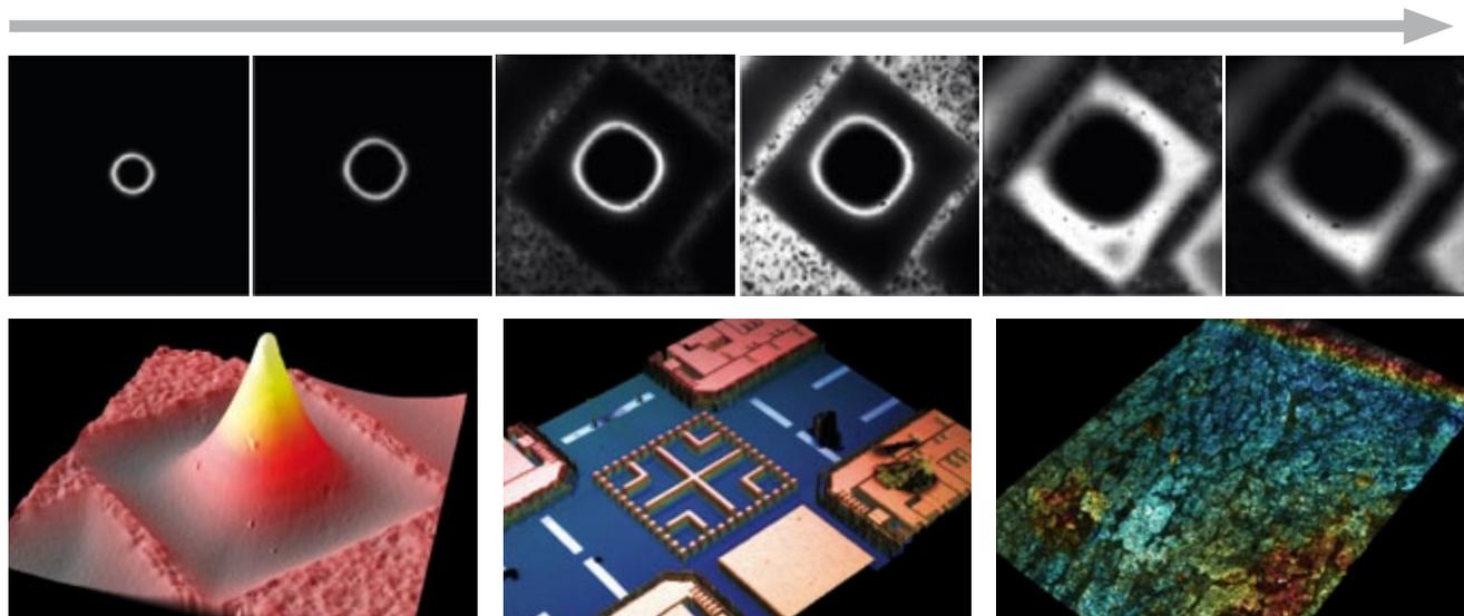
Steps of a confocal scan of a bump on a wafer surface
